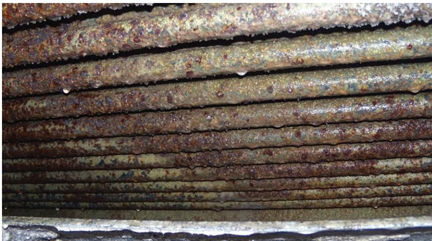
Scale can form thick deposits on heat transfer areas, reducing water flow, decreasing heat transfer and causing high head pressure.
