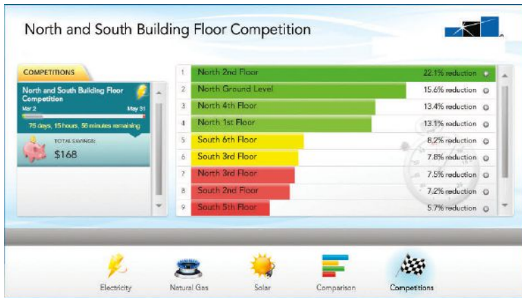
Figure 7: The use of submetered data can influence human behavior to reduce energy consumption, as shown in this example of the company headquarters floor-by-floor competition. Courtesy: Mortenson
