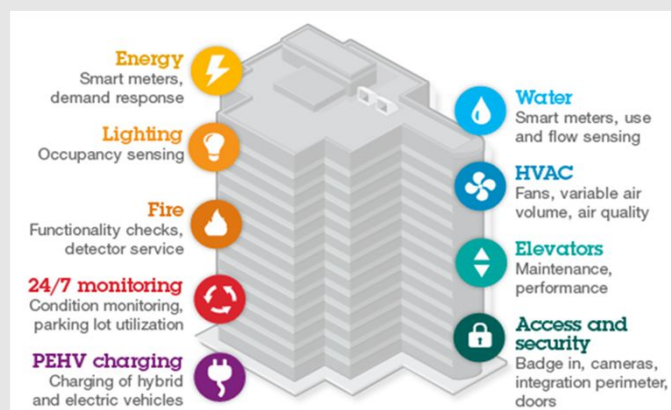
Figure 1: Scope of Smart Building
